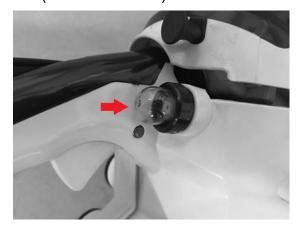
Pull the choke lever. It will close and the throttle will be moved to the starting position.
